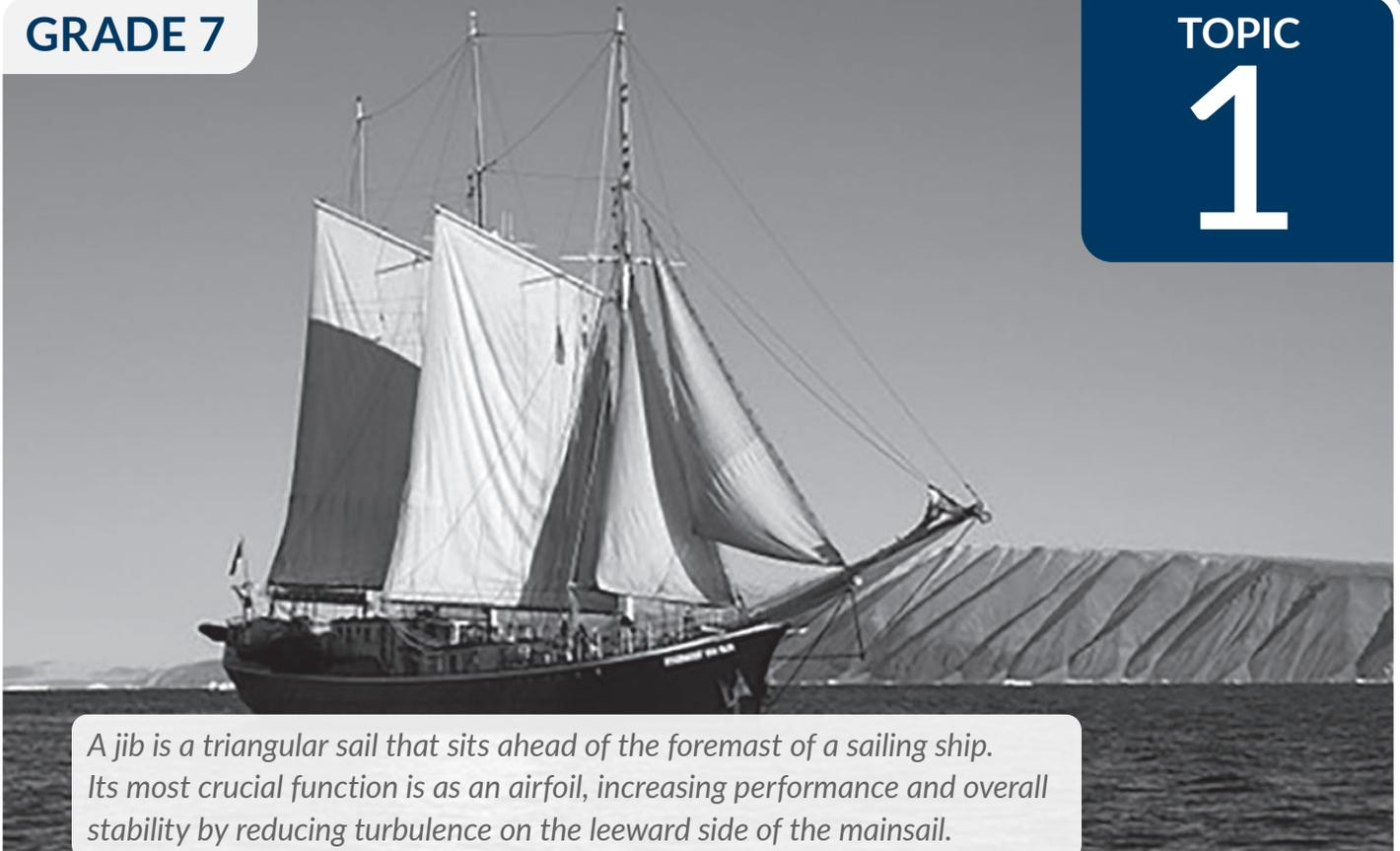
*A jib is a triangular sail that sits ahead of the foremast of a sailing ship. Its most crucial function is as an airfoil, increasing performance and overall stability by reducing turbulence on the leeward side of the mainsail.*
