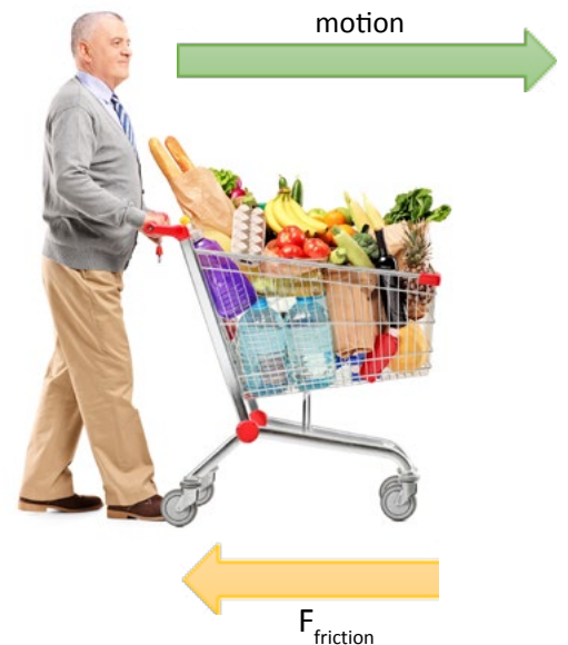
The force of friction is always in the opposite direction of the motion of the object.
