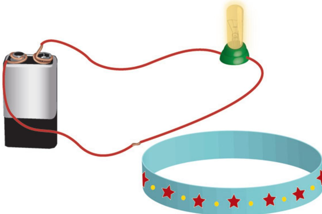
Electrical energy cannot travel through the circuit when the “door” is open. In the circus, the animals could not perform when the door was open or when the ring was incomplete.
