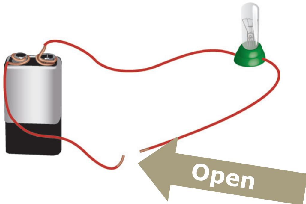
In this open circuit, the light is not working because the wires are not connected. Sometimes these circuits are called *incomplete* or *broken*.
